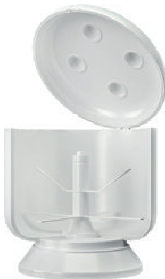
Schematic drawing of a high speed mixer used for PVC dry-blend preparation ("PVC compounding")
